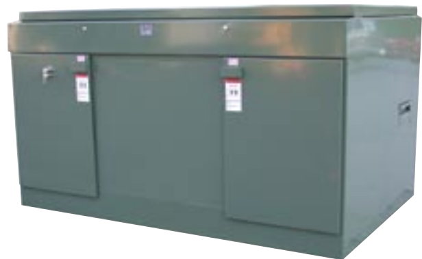
Figure 7. Exterior view of FP Primary Metering padmounted switchgear with incoming cable termination compartment at right and fuse compartment at left. Key interlocks on fuse-compartment door prevent opening the door unless the tap switch is open. Associated key interlock on switch-operating shaft of tap switch is captive when switch is closed and can't be removed until switch is open.
