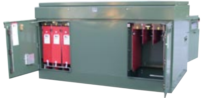
Figure 1d. Open door view of incoming bus-termination compartment (at right) and outgoing fused-feeder compartment at left with dual-purpose barriers in place. Independent compartment doors allow access control.
