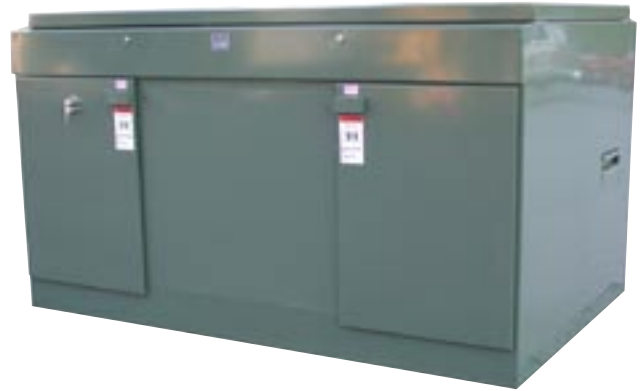
Figure 1c. Exterior view of unit with incoming bus-termination compartment on right and fuse compartment on left. Door on fuse compartment includes key interlocks to prevent access to fuses unless tap switch is open and to transfer block for connected transformers. Inset in Figure 1b shows the key interlock on switch-operating shaft behind access cover identical to that on the tap switch.
